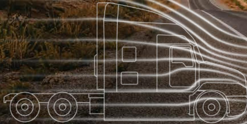
By displacing air to the sides, as well as over the hood and roof, Anthem cuts wind resistance and improves fuel economy by up to 3%. These aerodynamic fairings are at the core of the **Mack HE+ Package**, which arms an Anthem with the ultimate in fuel-efficient features.
